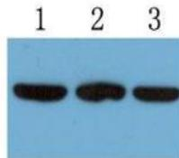
WB检测VDAC1 (MD10) 抗体, 抗原为HeLa细胞裂解物, 每个蛋清样品20  $\mu$ g, 抗体比例1: 1000 (1), 1: 2000 (2), 1: 5000 (3) 稀释
